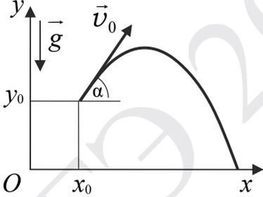
$\begin{cases} x(t) = x_0 + v_{0x}t = x_0 + v_0 \cos \alpha \cdot t \\ y(t) = y_0 + v_{0y}t + \frac{g_y t^2}{2} = y_0 + v_0 \sin \alpha \cdot t - \frac{gt^2}{2} \\ \begin{cases} v_x(t) = v_{0x} = v_0 \cos \alpha \\ v_y(t) = v_{0y} + g_y t = v_0 \sin \alpha - gt \\ \begin{cases} g_x = 0 \\ g_y = -g = \text{const} \end{cases} \end{cases} \end{cases}$ | -                                 | +                   |
